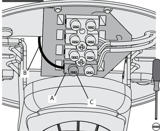
This is the procedure for steps 18-23. Thread the end of each wire into the terminal block (A) on the hanger bracket, then secure each supply main (B) by tightening the small setscrews (C).
