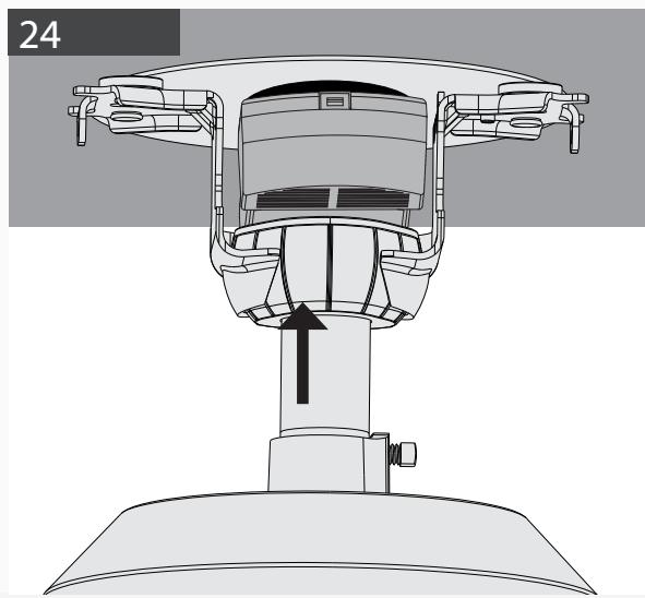
Place receiver in ceiling bracket. Excess wire may be placed into the outlet box for non-concrete ceilings or inside the hanger bracket for concrete ceilings.
