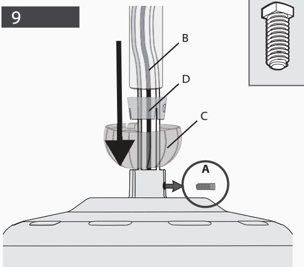
Remove the pre-installed setscrew (A) so that the downrod (B) can be inserted. Save the setscrew (A). Guide the downrod ball (C), sleeve (D), and downrod (B) down the wires coming from the fan.
