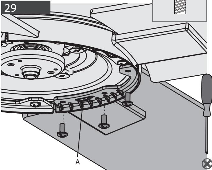
Lightly attach the blade arms to the motor with screws found in the X hardware bag, then securely tighten after both screws are attached.
