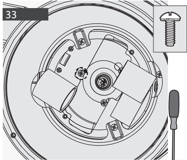
Insert a third light kit assembly screw, found in the hardware bag, into place and tighten all three screws securely.
