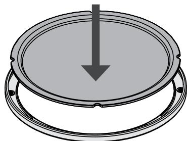
Align the globe indentations with the globe retainer screw holes and carefully lower the globe into the globe retainer until it rests in place.
