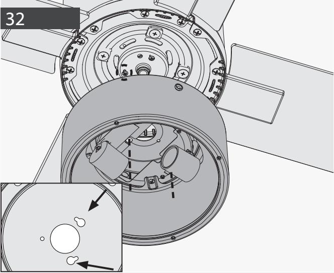
Align the keyhole slots in the top of the light kit assembly with the partially installed assembly screws. Wrap the keyhole slots around the screws and twist counterclockwise.
