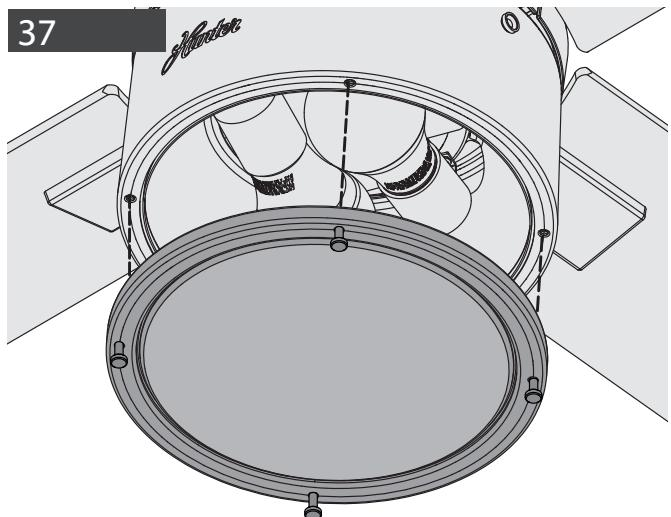
Lift the globe assembly and attach it to the upper switch housing using the four thumbscrews. Tighten all four screws securely by hand.
