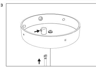
Lead the fabric cable in through the cable relief inside of the ceiling plate.
