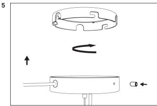
Attach the ceiling plate to the bracket by turning the ceiling
