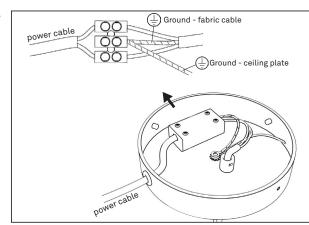
1. Lead the fabric cable into the cable connector. NB: After adjusting the length carefully reinsert the cables in same positions: Ground cable from ceiling plate and ground cable in the center of the cable connector.
