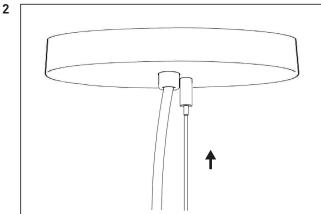
Press the wire through the wire lock to adjust the chandelier to the desired height.
