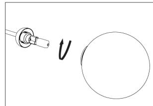
Take the glass globe and carefully place it over the light bulb and socket.
