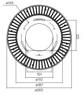
1 Keep the inner edge upwards 3 ø145 ROBY 2.6 & ROBY 3.5 have the same base plate 101 mounted. ø110
