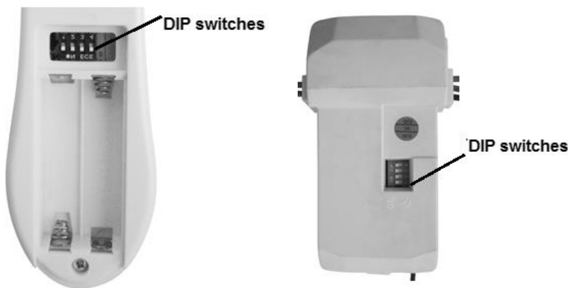
Fig. 10 Remote battery compartment
