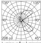
Luminous flux luminaire 2250 lm
