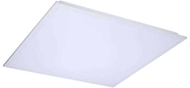
Quantum is a range of recessed integrated LED panels for general indoor lighting applications such as breakout areas, offices and meeting rooms. Max. drive current: 600mA; Max. power: 28W; Lifespan: 120.000Hrs L70:B50; 4000K; CRI 80; Efficacy up to: 161Lm/W; Fixture lumen: 4500lm; Lumen output using EM kit: ~500lm; Glare control <19; IK03; IP54 (from the front); Class II; DALI dimmable. Tp(a) rated diffuser that self-extinguishes within 5 sec when a flame has been removed.
