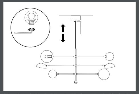
6. Unmount the screw from the small metal ring underneath the ceiling cup, then gently pull down the cable (Never pull the cable, while the screw is fastened in the cable). When the height is adjusted, please fasten the screw to the small metal ring underneath the ceiling cup. When adjusting the cable length always make sure that the cable is held straight and is not twisted as it can damage the fabric cable.
