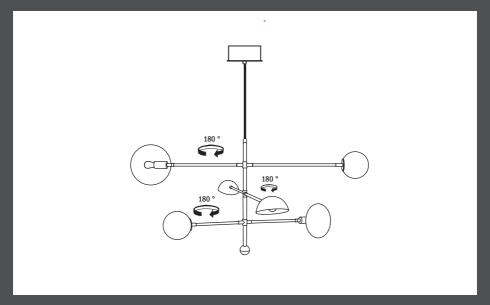
5. The lamp is designed to only rotate up to 180 degrees from its original position. This means that you cannot turn the lamp beyond 180 degrees and it is restricted by the maximum 180 degree rotation range. Going beyond this limit is not allowed and will cause damage to the lamp. In the process of adjusting the lamp, please adjust the upper and lower poles in order to achieve the effect of the balance of the lamp.
