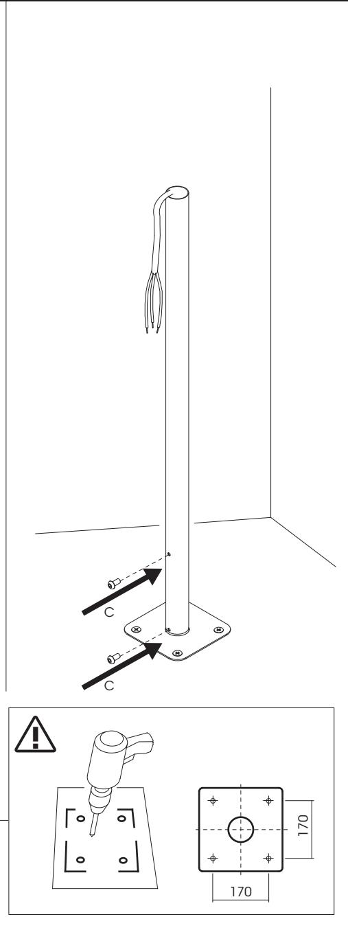
**BELLHOP Ø200 - POLE:****FISSAGGIO CORPO LAMPADA - FIXTURE FASTENING**
