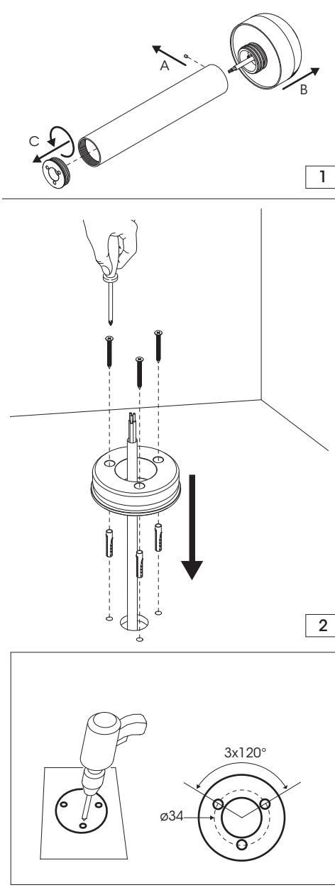
**BELLHOP Ø125 - BOLLARD H.380-850mm: FISSAGGIO - INSTALLATION**
