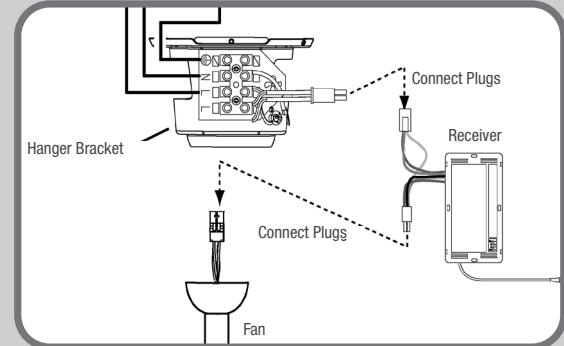
Before installing the Universal Remote Control Receiver, use the pull chains to set the fan speed to HIGH and the light to ON. Be sure power is OFF before proceeding with installation.
