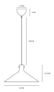
Voltage (V): 220-240 Volt IP degree: IP20 Maximum bulb wattage (W): 60 Class (Class 1, Class 2, Class 3): Class 2 (Double isolated) Socket type: E27 Parallel connection: False
