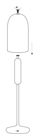
Mount the shade onto the base, and screw back the 3-way-touch-switch to fix the shade
