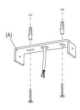
Mount the ceiling mounting to the ceiling with two appropriate screws and plugs. Always use correct screws and plugs for the mounting surface.
