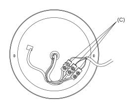
3. Connect the electrical cable with the terminal strip (C).
