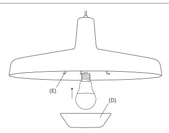
To insert the light bulb, release the undershade (D) by pressing three undershade brackets (E) inwards.
