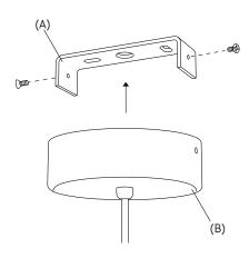
1. Remove the ceiling mounting (A) by unscrewing two screws from the lamp body (B).
