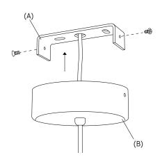
4. Attach the lamp body back to the ceiling mounting.
