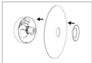
Carefully place the cover plate over the socket. Afterwards place the small metal plate over the socket.
