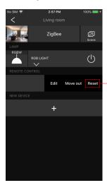
From your ZigBee controller or hub interface, choose to delete or reset the remote as instructed, indicator flashes 3 times quickly to indicate successful removing.
