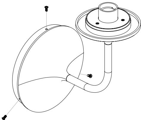
**5.** Assemble the shade by screwing it onto the base,
