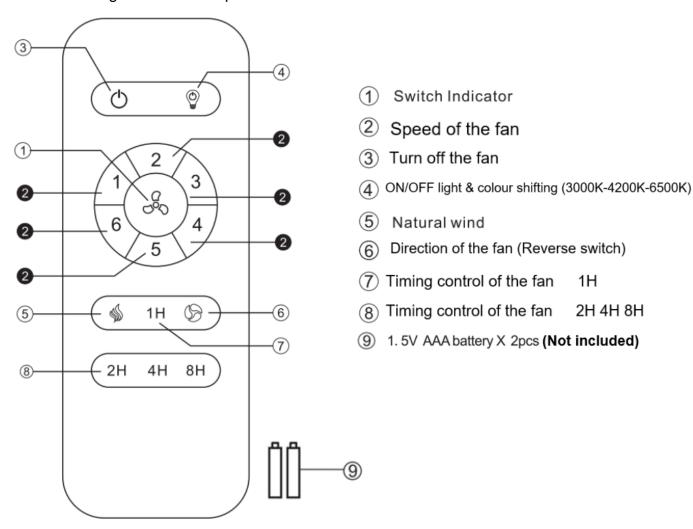
The remote has memory function. If the fan or light is turned off by the isolating switch over 7 seconds, the next time to turn on the fan or light will be on last setting.
