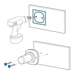
3. Firmly screw the knob of the mounting bracket into the mounting hole.
