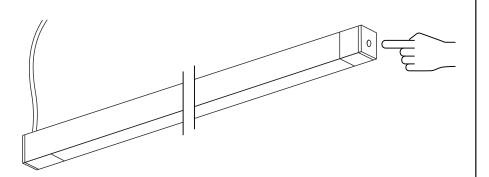
Remember to set the correct colour temperature **before** installing the spot lights
