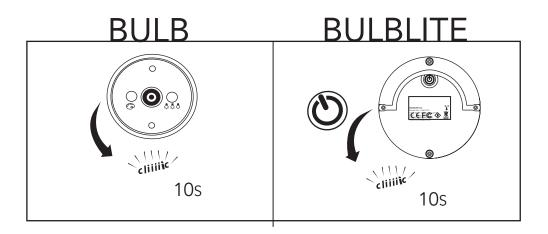
A procedure can be used to restart the products. If the user loses their smartphone or a device is not working properly for some reason despite a properly charged battery, simply follow the procedure below to restore the device to factory settings (it will also probably be necessary to delete the device causing the issue in the device listing in your smartphone's application. Please refer to the additional functions for this procedure).
