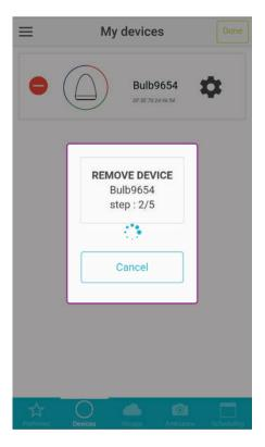
When a device is removed from the Bluetooth mesh network you should see it flashing briefly in red, a delete message appears on the screen of your smartphone then the module disappears from the device list.
