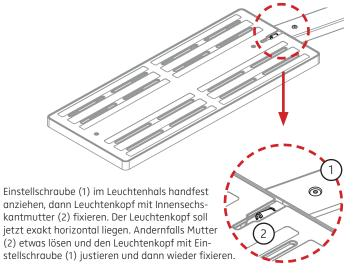
Fasten setting screw (1) on top of the tube hand-tight, then fix the head using the hexagon nut (2). The luminaire head should now be aligned horizontally. Otherwise slightly release the nut (2) and adjust the head by means of the setting screw (1). Fix it again.
