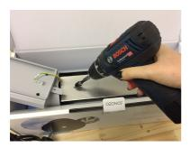
3. Put the outer case aside and unscrew the screw of the inner case.
