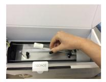
5. Now lift the lamp first on the left, then on the right side out of the bracket and carefully pull the lamp out of the plug.
