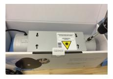
2. Unscrew the two screws with a Torx IO screwdriver.
