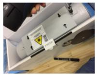
10. Close the outer case and retighten the screws left and right.
