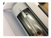
6. Take the new lamp and insert it into the plug completely.
