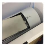
9. Reassemble the inner case. Start by inserting the inner case as far to the right as possible and then slide it to the left. Now retighten the screw to fix the inner case.
