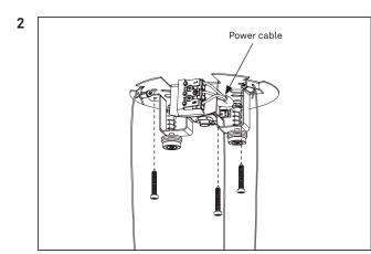
Lead the power cable through the mounting bracket and attach it to the ceiling.
