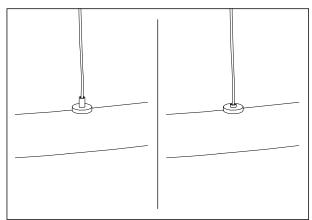
Use the wire locks on the ring to adjust the lamp to its final position. It is recommended to use a spirit level.
