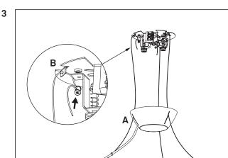
Adjust the suspension wires close to its final position by loosening the wire lock and leading the wire through.
