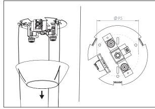
Pull the cover plate away from the mounting bracket. It is attached with strong magnets and might require some force.
