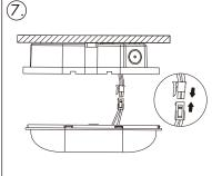
Connect the plug of the LED-module to the socket of the luminaire housing. Press the cover of the LED-module evenly onto the lower part of the luminaire until the clips provided snap into the connection points.
