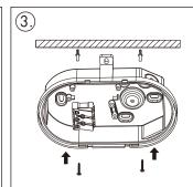
Use the backboard or legs as a template in order to mark and drill the appropriate fixing holes on the ceiling/wall. Secure the backboard with backboard or legs with raw plugs and screws on the ceiling/wall.
