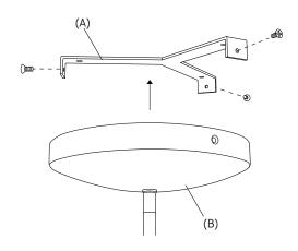
1. Remove the ceiling mounting (A) by unscrewing three screws from the lamp body (B).
