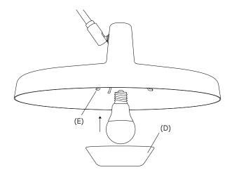
5. To insert the light bulb, release the undershade (D) by pressing three undershade brackets (E) inwards.
