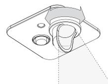
The detection range of the motion sensor can be limited by a cover. By twisting the cover the range desired can be chosen.
