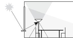
2. Do not expose the sensor to direct sun light. In the window area the sensor should be placed in such a way that the entire coverage zone is included within the said space and so as to avoid that the reflections of the daylight, which result from reflecting surfaces, fall into the sensor. Note: reflections on glass or metal surfaces might cover the sensor and, as a consequence, affect the lighting control. Therefore, the sensor must be absolutely displaced.
