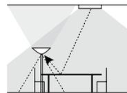
1. Do not expose the sensor to direct light. The reflected light will be detected at the workplace by the ambient light sensors. For this reason, you must avoid locating the sensor in a place where it might be directly illuminated by a light source.
