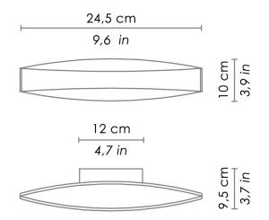
Wall lamps with a matt white painted aluminium frame and a transparent polycarbonate diffuser. The product is suitable for indoor use only.
