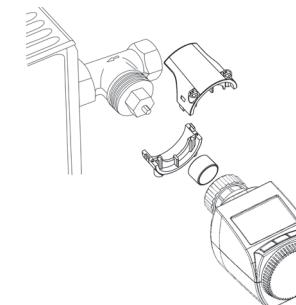
The figure on the right shows another view of how device is mounted on the radiator.
