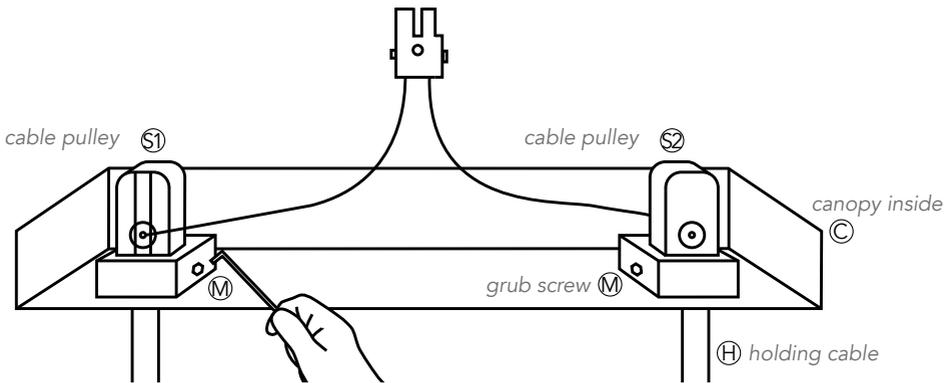
Because wood is a natural product, each piece of wood can vary in density. The weight of every HerzBlut lamp body ① could be different. The counter weight ② is set up for an average weight. When the lamp body ① heavier is as the counter weight the “extra weight” has to be counter balanced.
