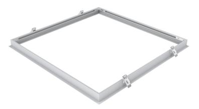
Plasterboard ceiling frame accessory for panels 625x625mm. Suggested cut-out size 655x655mm. Suitable ceiling thickness 15-40mm.
