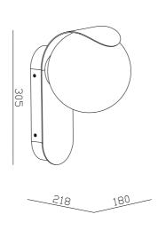
Voltage (V): 220-240 Volt IP degree: IP44 Maximum bulb wattage (W): 10W Class (Class 1, Class 2, Class 3): Class 1 (Earth contact) Socket type: E27 Parallel connection: True
