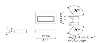
Wall-ceiling lamp with a matt white, dark grey or corten painted die-cast aluminium frame and a polycarbonate diffuser. The high IP rating (IP54) makes the lamp ideal for indoor and outdoor use.
